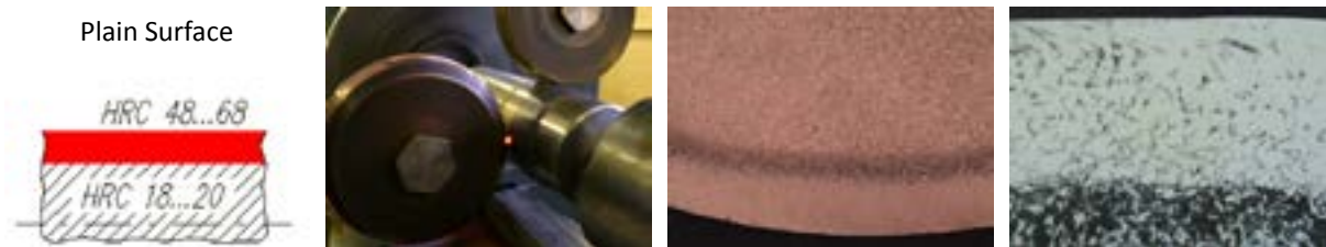
Electromechanical surface quenching of the drill pipes outside surface.
